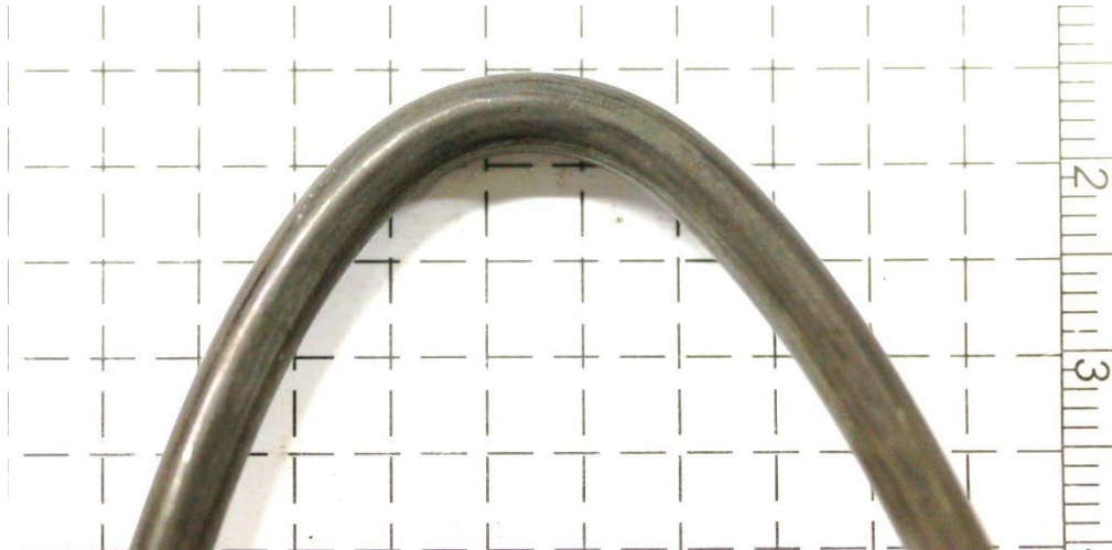
Figure 12 Typical Wire After Bending
