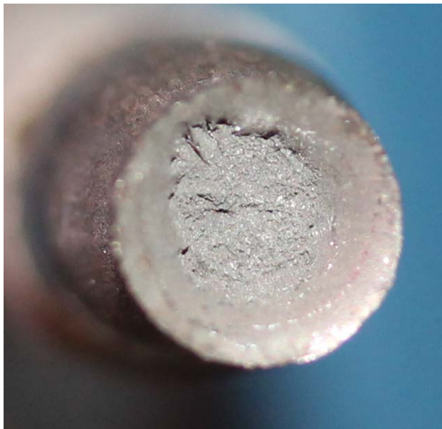
Figure 54 Typical Fracture Surface (3/4)
