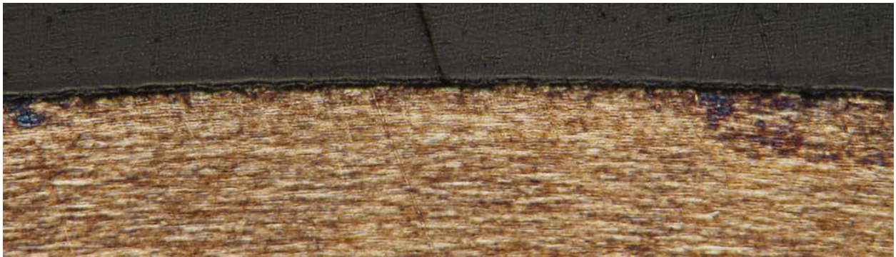
Figure 58 9-Month SSK Wet Exposure Sample - Etched with Nital (Field Width- 2 mm)
