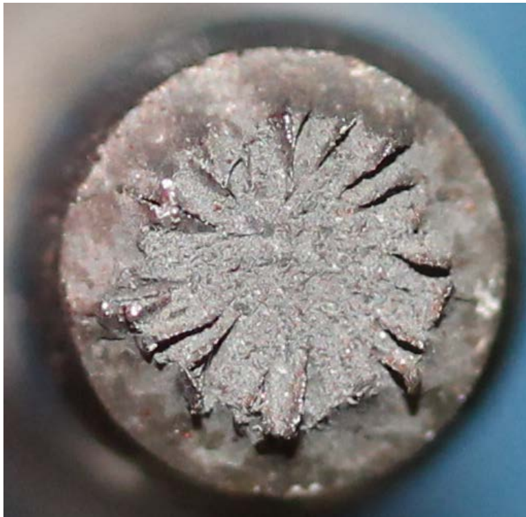
Figure 52 Typical Fracture Surface (1/4)
