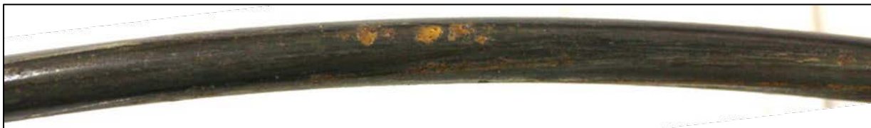
Figure 31 Outer Wire of 9-Month SSK Wet Exposure Sample - Before Bending (2/3)
