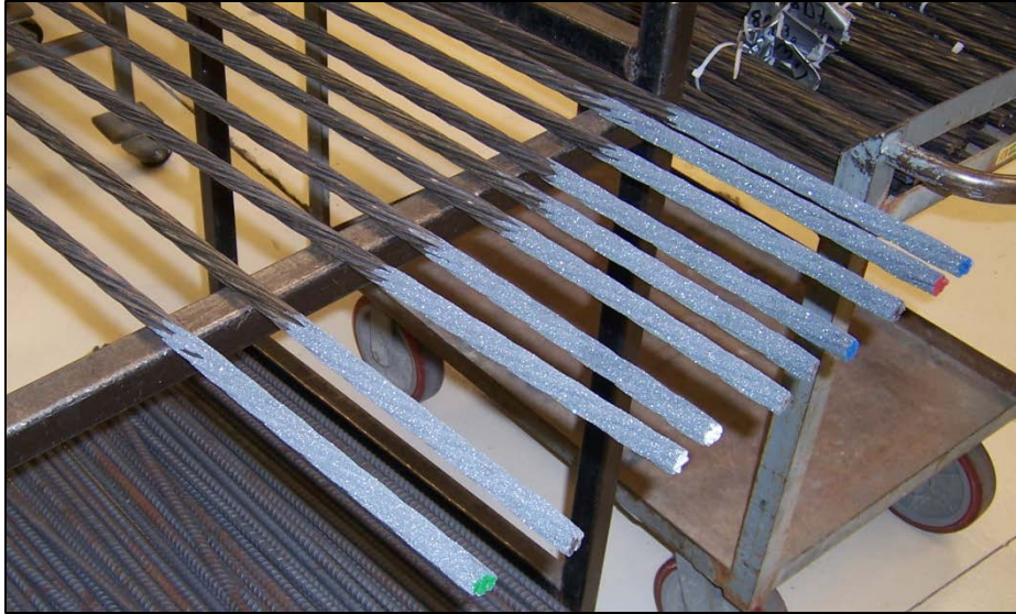
Figure 35 Sample Strands' Ends Coated in Grit Material Awaiting Tensile Testing
