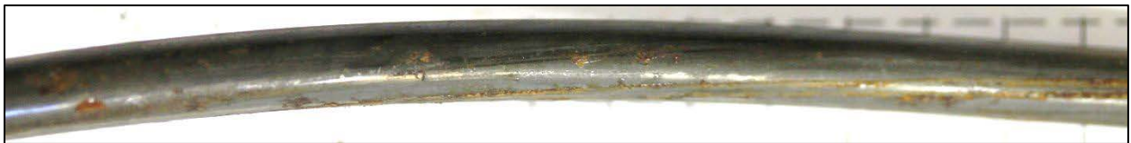
Figure 32 Outer Wire of 9-Month SSK Wet Exposure Sample - Before Bending (3/3)
