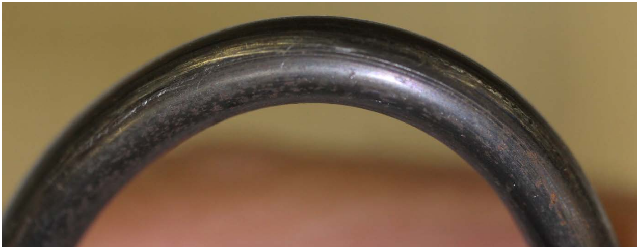
Figure 61 8-Week SSK 2-Open Exposure Sample - Exterior of Bend Surface
