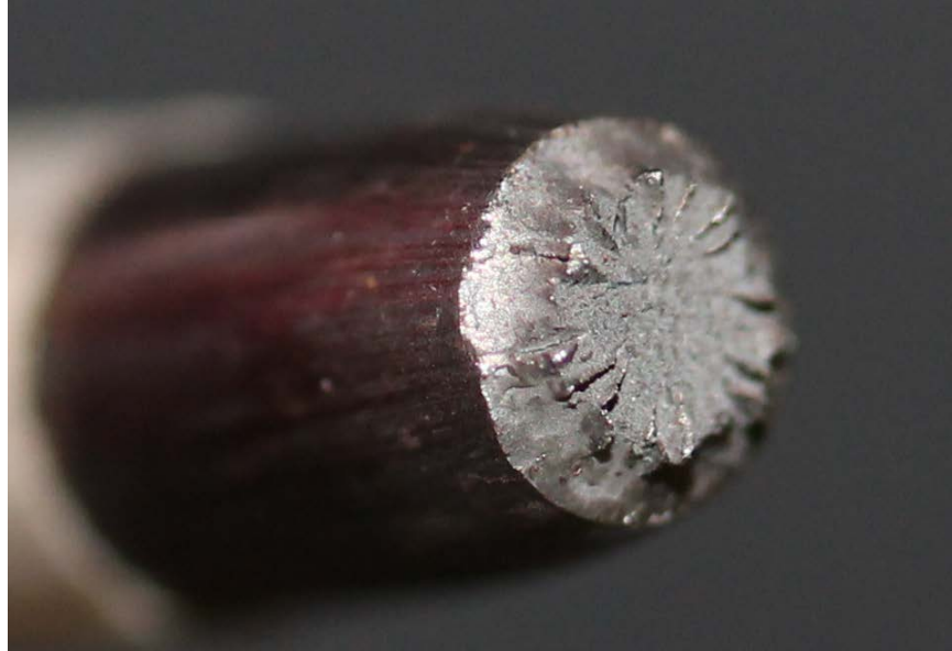
Figure 53 Typical Fracture Surface (2/4)
