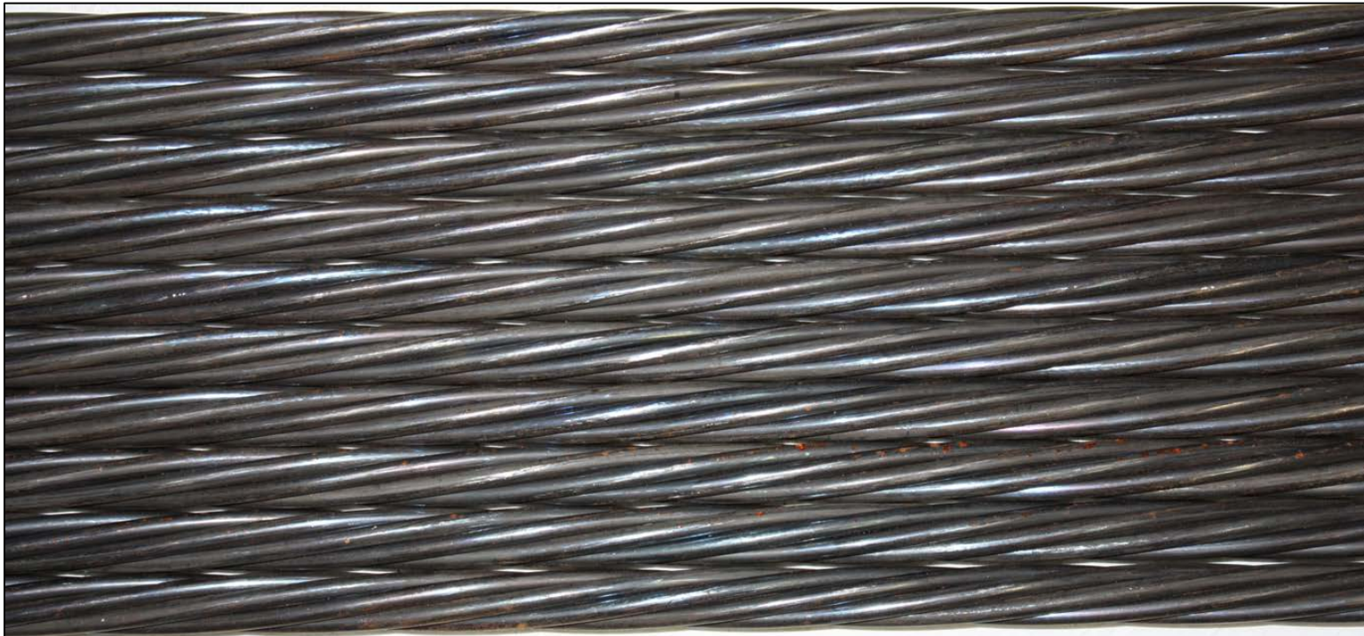
Figure A1.71 Typical As Received Condition of Strands Prior to Exposure
