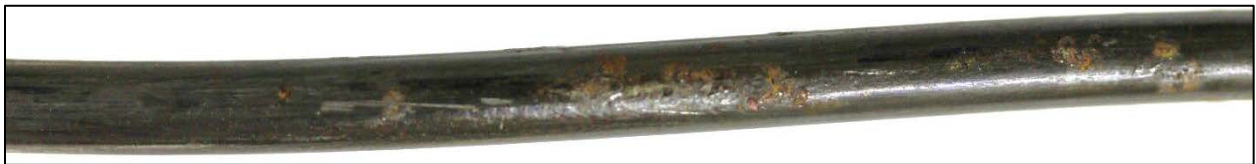
Figure 30 Outer Wire of 9-Month SSK Wet Exposure Sample - Before Bending (1/3)
