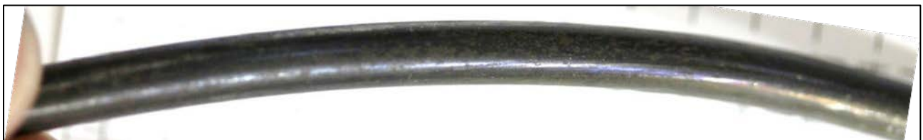
Figure 33 Outer Wire of 8-Week SSK 2-Open Exposure Sample - Before Bending
