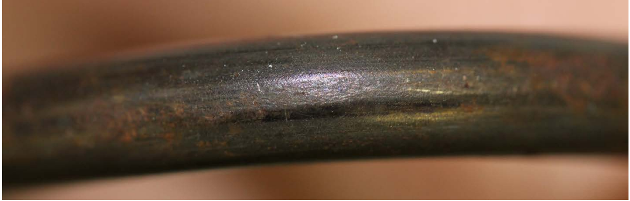
Figure 56 9-Month SSK Wet Exposure Sample - Exterior of Bend Surface
